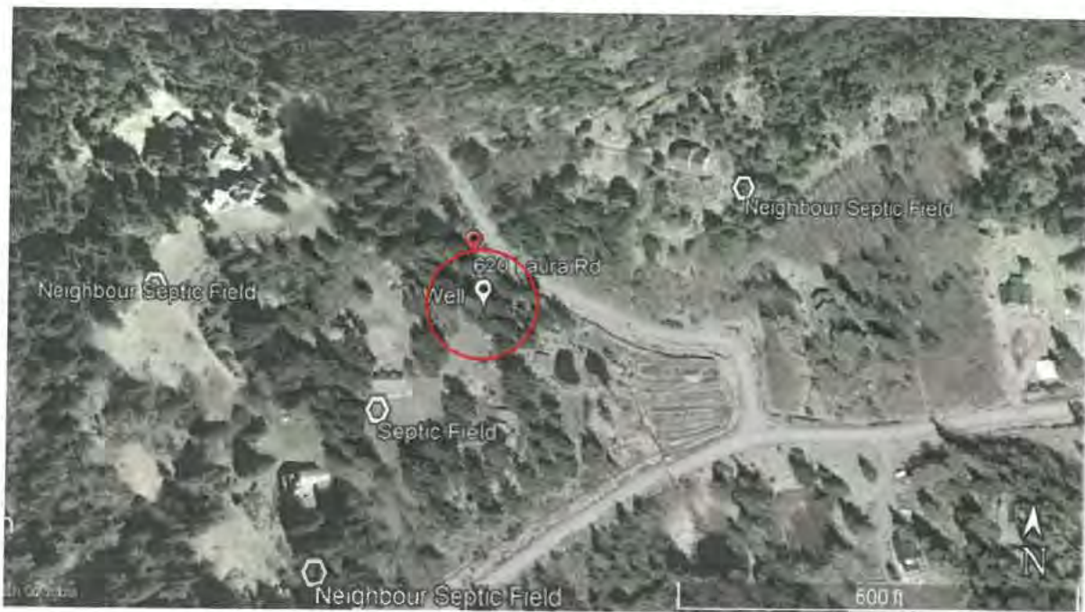
Figure 10. Location of well in relation to on site and neighbouring septic fields (onsite sewerage systems). Red circle shows approximate 30m radius from well. Sewerage System Regulation mandates 30m setbacks of onsite sewerage systems from water wells. Image source: Riley's Cidery.
