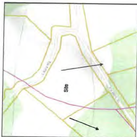
Figure 7. A drainage divide runs through the Site at the NW side (purple line). Most of the site drains to the south toward Killamey Creek (see Fig.6). The northwest portion of the Site drains to the southwest, ultimately to Turnstall Bay.
